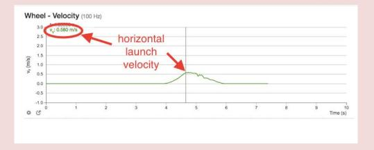
time of flight of projectile t= \_\_\_\_  $\pm$  \_\_\_ calculated from  $t=\sqrt{\frac{2h}{g}}$  range  $R_{theoretical}=$  \_\_\_  $\pm$  \_\_\_ calculated from R=vt
